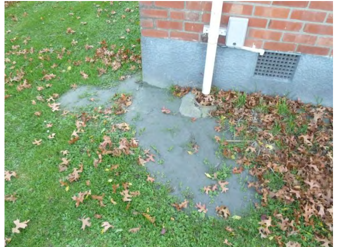
d) Isolated area of liquefaction ejecta on lawn
