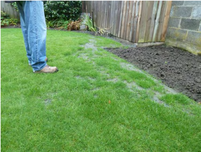
c) Isolated area of liquefaction ejecta on lawn
