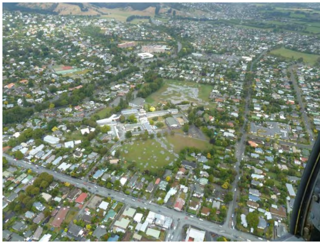
a) Aerial photo of liquefaction ejecta at Cashmere High School
