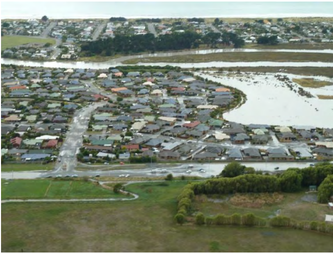
m) Aerial photo showing liquefaction ejecta on Seabreeze Close
