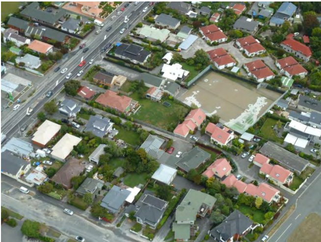
i) Aerial shot of Redcliffs with liquefaction ejecta
