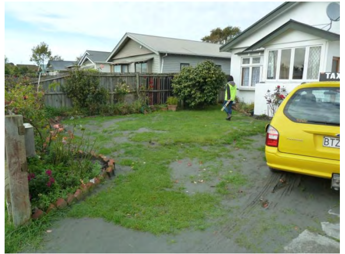
n) Liquefaction ejecta on lawn
