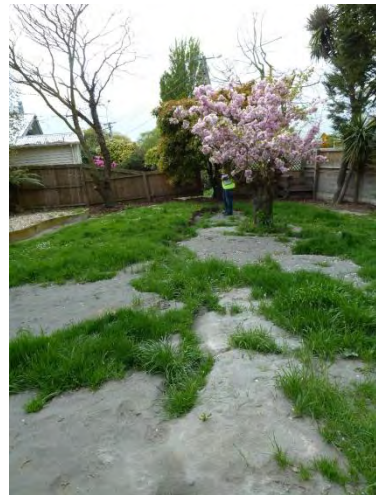
d) Numerous patches of liquefaction ejecta
