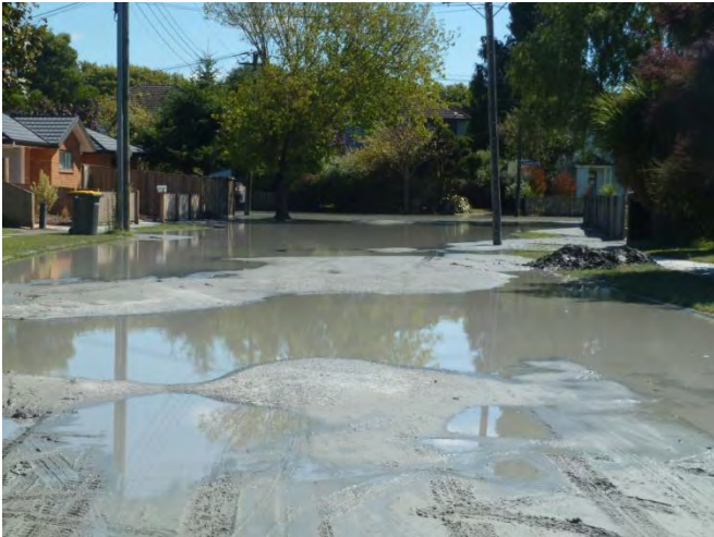
o) Road damage on Orontes Street with ponding water
