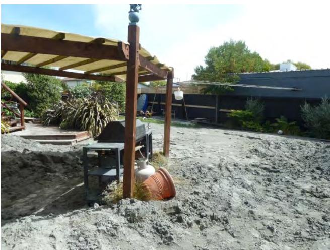
k) Liquefaction ejecta around property
