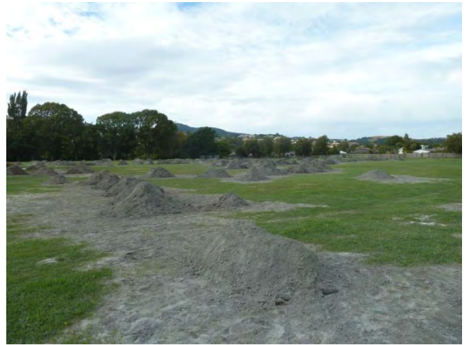
n) Liquefaction ejecta piled on Cashmere High School lawns
