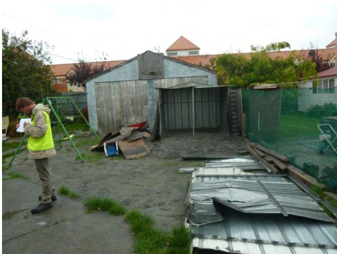
k) Large area of liquefaction ejecta on lawn
