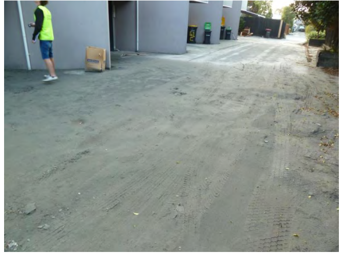
b) Liquefaction ejecta covering driveway
